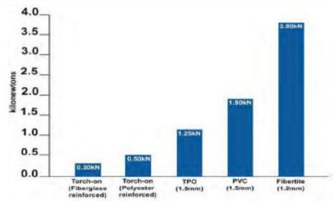
FiberTite's standard membrane (thickness 1.2mm) has five times the puncture resistance of 4mm bitumen based torch-on membranes. To quote the scientists at FiberTite – thicker isn't better, BETTER is BETTER. And as FiberTite membranes increase in thickness (1.5mm - 2.3mm) the fabric reinforcement gets stronger still, until, quite literally, their puncture resistance goes off the scale.
